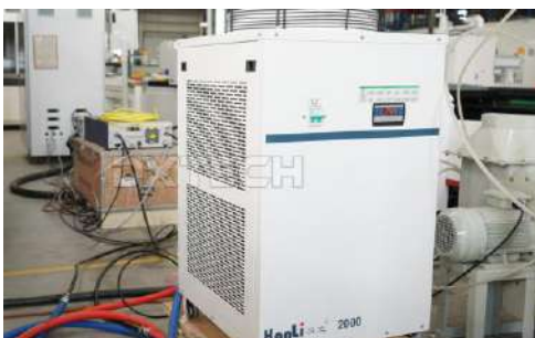
Hanli water chiller
